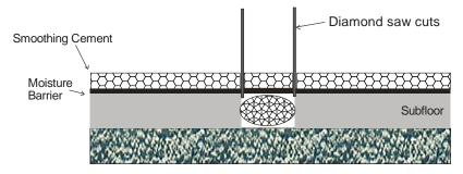
As per step 29 the material from the saw cut has been removed.
