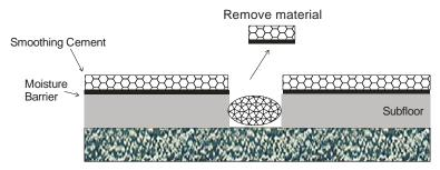
As per step 30 Moisture Barrier is painted thoroughly down into the joint. A suitable flexible sealant system is then installed (may include mouldings or metal extrusions
