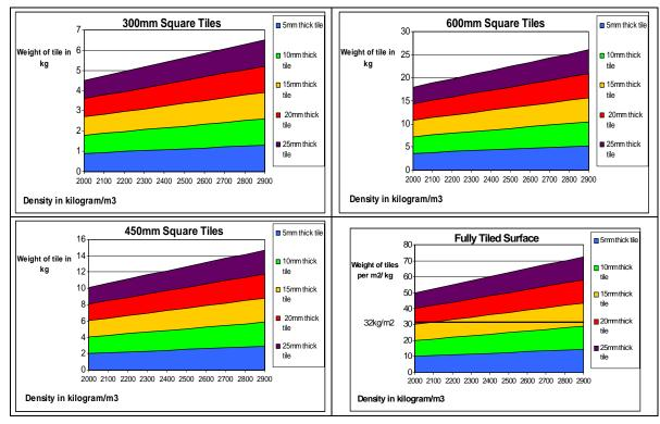
A typical 400mm x 400mm fully vitrified tile or ceramic tile would be limited to a thickness of about 10mm to be within the 32 kg per m² limit. Care should be taken when assessing agglomerate and natural stone tiles as the bulk density of stone tiles can range from 2300kg/m³ to 3200kg/m³ depending upon the composition.
