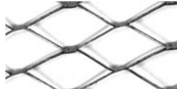
An example of E-glass\* fibreglass matting with 10mm apertures and 2x 0.75mm thick fibres.
