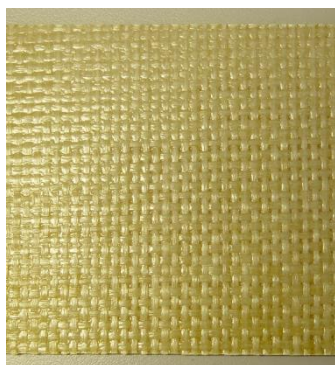
Mesh backed tile with the mesh fully embedded in resin. Epoxy resins are difficult to bond to, whilst polyester resins can be attacked by C class tile adhesives.
