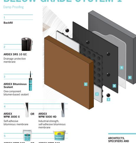
ARDEX WPM 240 Solvent-based bitumen **ARDEX WPM 247**
