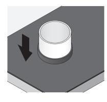
After pulling pipe down tape upstanding WeldTec™ to pipe using WeldTec™ Detail Tape. Finish with stainless steel clamp.
