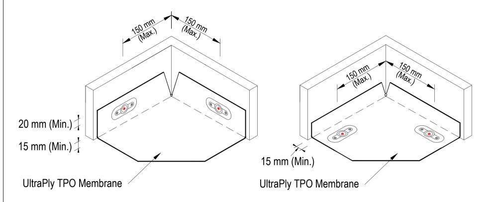
Note: Base Flashings and Terminations are not shown for clarity.
