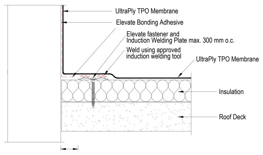
Induction Welding Plate must be at least 25 mm away from angle-change but not more than 150 mm
