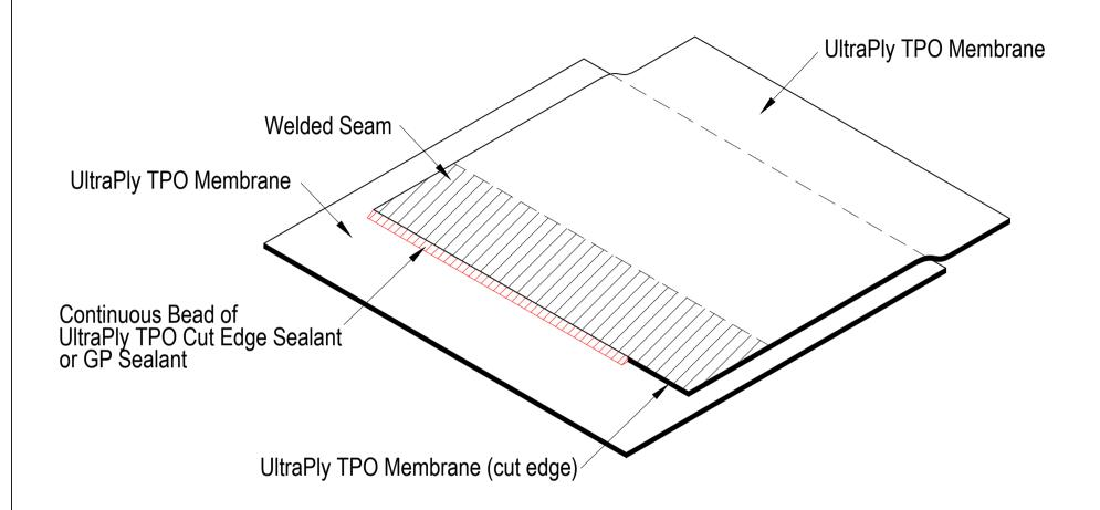
Note: When polyester reinforcement of TPO is exposed, apply Cut Edge or GP Sealant to entire exposed edge.
