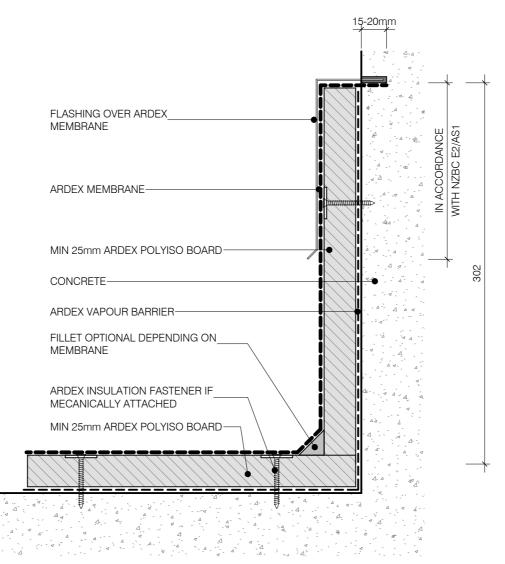
NOTE: ARDEX MEMBRANE IS ADHERED WITH ADHESIVE UPTO THE CHASE. THE FLASHING IS SEALED INTO THE CHASE USING ARDEX CA20P OR ARDEX RA88.
