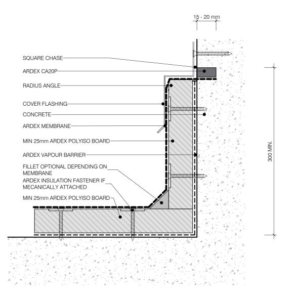
NOTE: ARDEX MEMBRANE IS ADHERED INTO SQUARE CHASE AND FINISHED WITH ARDEX CA20P SEALANT
