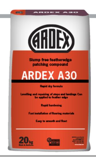
ARDEX A 30 is a slump free feather edge patching compound that is designed for internal filling of cavities, holes, unevenness and patching work in wall and floor areas. When mixed with water the result is a smooth slump free mortar with a pot life of approximately 15 minutes. ARDEX A 30 dries fast through hydration to a virtually tension free compound.
