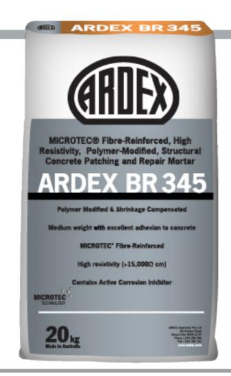
ARDEX BR 345 High Resistivity Structural Concrete Patching and Repair Mortar is designed for reinstating concrete surfaces damaged through concrete spalling and other chemical or mechanical causes. ARDEX BR 345 is a high-build patching mortar and can be applied up to a thickness of 80mm on vertical, horizontal and overhead surfaces. It is designed to be used for applications where high resistivity of the mortar is required.
