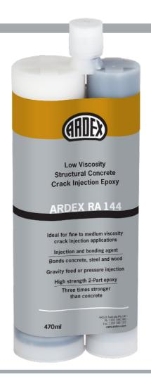
ARDEX RA 144 is a low viscosity, high modulus structural epoxy adhesive used for a variety of repair projects. With its low viscosity, it is perfect for horizontal gravity-feed repair of fine to medium size cracks and can be used in temperatures between 10°C and 35°C. Its bonding and sealing capabilities for interior and exterior slabs are exceptional.
