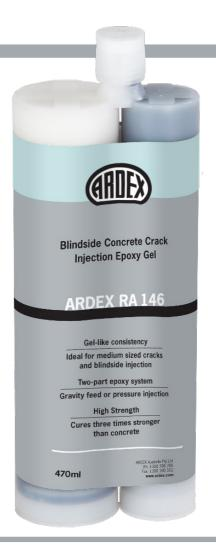
ARDEX RA 146 is a thixotropic structural epoxy adhesive system with a gel-like consistency for repair of medium size cracks when using an injection port system. ARDEX RA 146 is multi-viscous and flows like a liquid while under pressure and will cease flowing when no pressure is being applied. It is a high strength epoxy system perfect for blind-side crack repair of most substrates. It will bond the structure back to its original monolithic strength.
