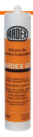
ARDEX SE is an acetic cure silicone sealant which is ideal for use in tiling applications due to the superior bond achieved when being used with glazed surfaces such as ceramic tile. Due to its high elasticity, ARDEX SE is able to accommodate movement up to 25% of the original joint width. It is exceptionally easy to apply and smooth, curing to form a permanently elastic, waterproof and dustproof joint seal.
