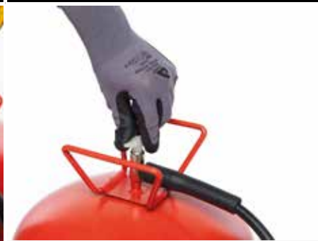
Turn the white valve of the canister counterclockwise until open. Do not close the valve until the canister is empty (this is to prevent the adhesive curing in the hose and gun).
