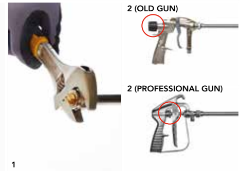
Make sure the spray gun tip is positioned straight and is tightened (1) and the adjustment screw is closed (2).
