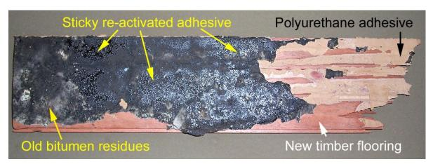
The above picture shows a sample of the 'blown' floor with the various features highlighted. Areas of the bitumen that were re-activated were quite sticky and weak. The Arditex layer was so thin that it does not show in the picture, but is present between the bitumen and polyurethane adhesive.
