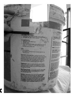
An example of a home made gauging bucket, which can result in variable or inaccurate water dosages unless carefully cut and used.
