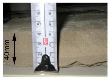
An example of material used above recommended thickness. In this case the product is ARDEX A45 used above the recommended maximum thickness of 20mm without a filler aggregate.
