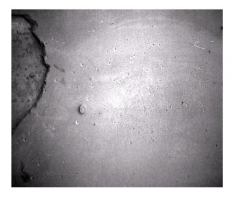
Where priming is not done on porous surfaces ant holing will occur. This is not satisfactory for vinyl flooring.
