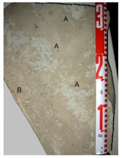
The floor shown on the left was particle board timber which was not sanded to remove the waterproof coating and building contaminants including plaster residues. This floor had also been rain affected and had a weak surface layer.
