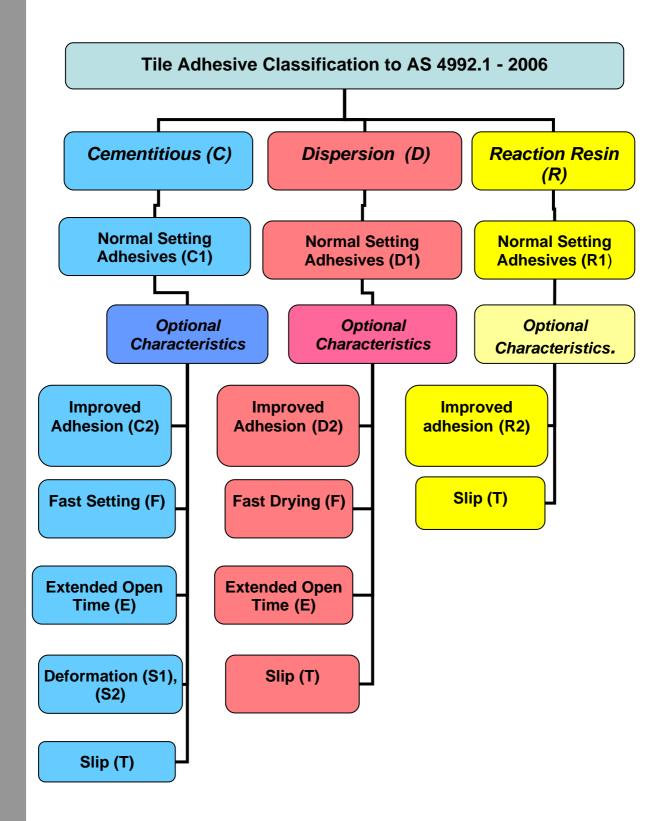
Performance characteristics may be different for each classification so it is important to correctly identify the type of adhesive being considered. With the confusion possible by using common descriptive names such as *rubber* adhesive or *organic* adhesive, correct identification ensures the required level of performance is provided.
