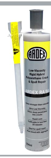
ARDEX RA 56 is an ultra-low viscosity, 2-component hybrid polyurethane adhesive. It is a rapid curing concrete repair material used when minimal down time is crucial. Its low viscosity offers deep penetration into hairline cracks for a structural repair. The addition of dry, bagged aggregate makes a quality spall repair product that is ready for grinding and open to traffic in less than 1 hour.
