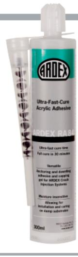
ARDEX RA 84 is a two-component, non-sag, styrene-free, acrylic system used for anchoring and dowelling applications in uncracked concrete using threaded rod and rebar. Due to its ultra-fast cure time, it is an ideal capping gel for ARDEX Crack Injection applications. ARDEX RA 84 is moisture insensitive, and can cure in damp, water-saturated environments.
