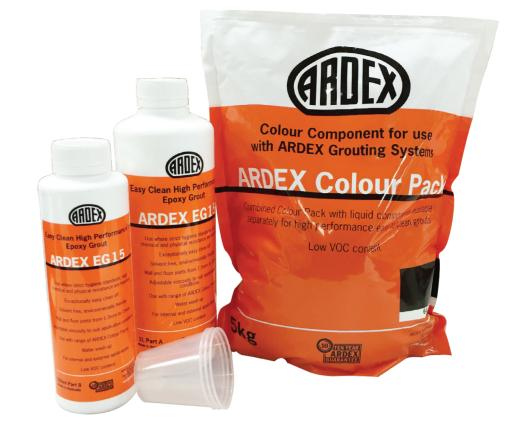
ARDEX EG15 is a high performance epoxy grout designed for situations that require strict standards of hygiene, high chemical and physical resistance. ARDEX EG15 is exceptionally easy to clean up during application. It can be used in joints up to 15mm wide on walls and floors.
